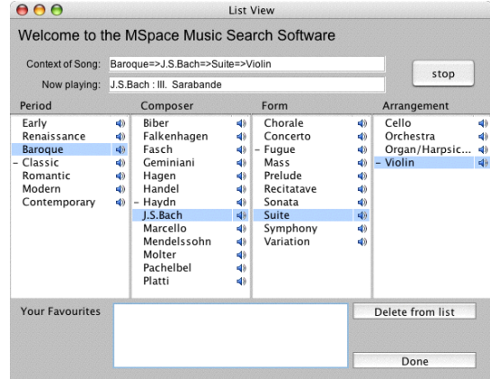
Figure 3: An mSpace multipane browser, viewing a database of classical music. The columns, from left to right, are Period , Composer , Form , and Arrangement . Each column corresponds to a level in a tree of choices. The children of the root node are in the left-most column, and leaves are in the right-most column. Selecting an item in every column corresponds to specifying a path through the tree. The left-to-right ordering of columns may also be changed, changing the structure of the tree, thereby allowing many possible trees to be browsed.
