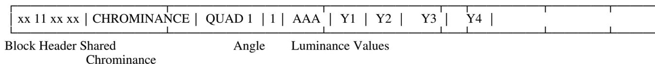
Figure 8. Format of an Extended LTC Quadrant
