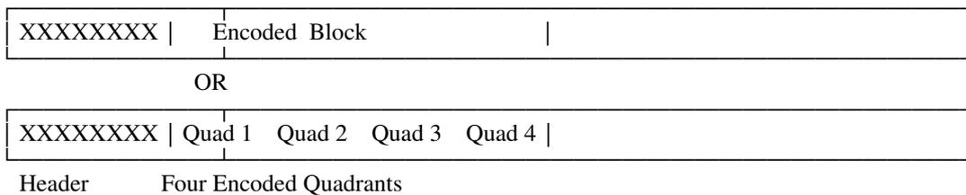
Figure 2. Format of an Encoded Block Decomposed into Quadrants
