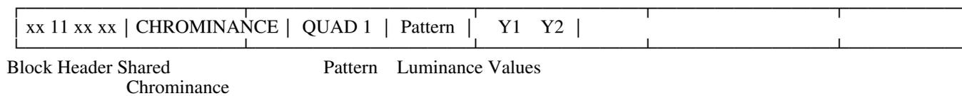
Figure 7. Format of a Statistical quadrant
