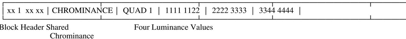
Figure 10. Format of Block with Sub-4 Quadrant
