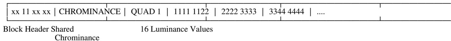
Figure 11. Format of Block containing a 16-luminance quadrant
