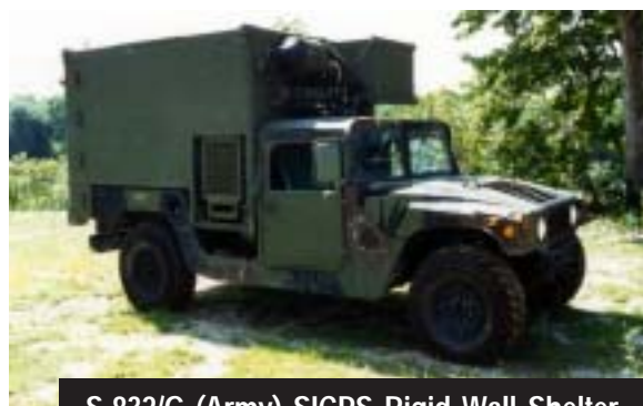
S-832/G (Army) SICPS Rigid Wall Shelter
