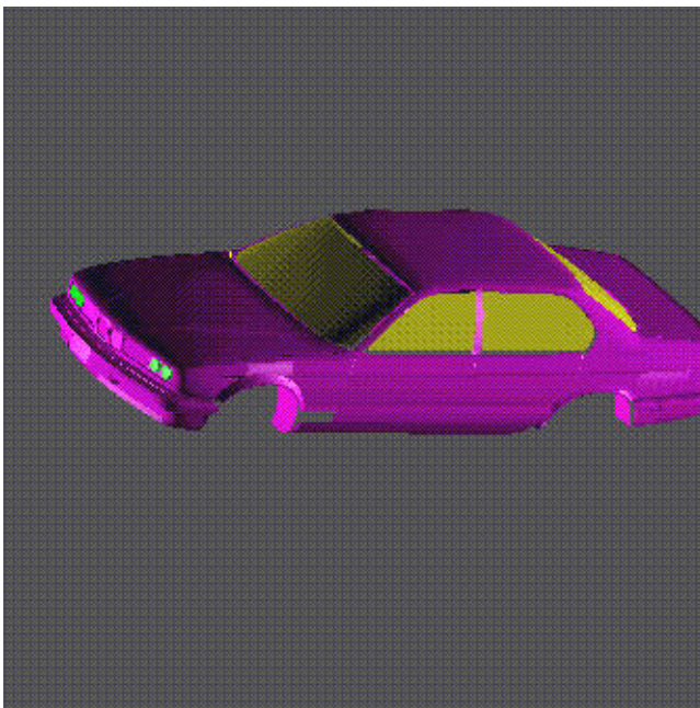
Figure 8. Shaded-lighted image (2 directional lights) (data courtesy of Csisgraph Corporation) has 77420 triangles, 526235 pixels, and was rendered in 0.29 seconds.
