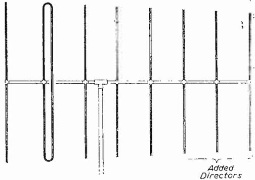
Fig. 4.—Adding directors to a yagi array.
