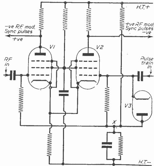
Fig. 10.—Pulse mixing stage.
