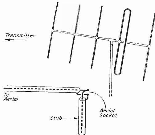
Fig. 5 (Top).—Tilting the aerial. Fig 6 (Bottom).—Using a stub.
