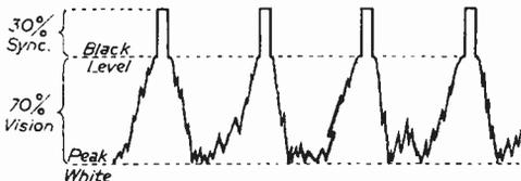
Fig. 1.—Video and sync waveform at the tube cathode.
