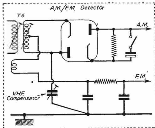
Fig. 2a.—Details of AM/FM detector.
