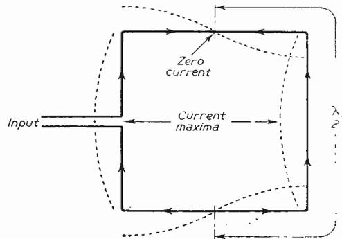
Fig. 2.—Current distribution around the loop.
