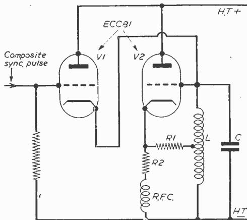
Fig. 8.—Oscillator and keying stage.
