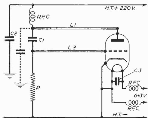
Fig. 1.—The theoretical diagram of the oscillator.
