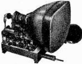
Latest improved circuits. Higher E.H.T. (brilliant picture). Improved sensitivity (for greater range). Chassis is easily fitted into any cabinet. 17" rectangular tube on adapted chassis. Less valves. 12 months' guarantee on tube. 3 months' guarantee on valves and chassis. With Valves. £25 19/6. Valve line-up 6SN7G, 6V6, EY51, 2-3D2s, EL33, EL14 and 7-6F1s. Turret tuner. 50" extra. Spare B.C.C. channel supplied at 7/6
