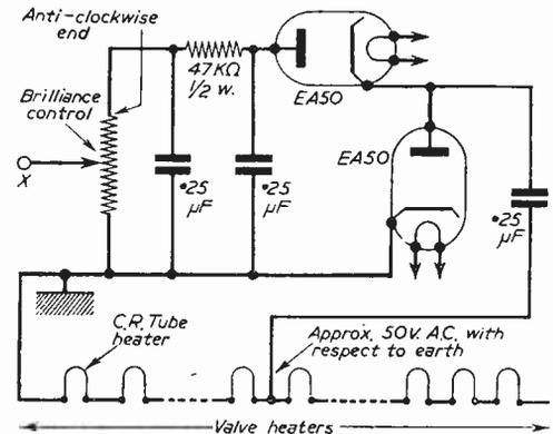
Fig. 2.—Bias line derived from the heater chain for brilliance control.
