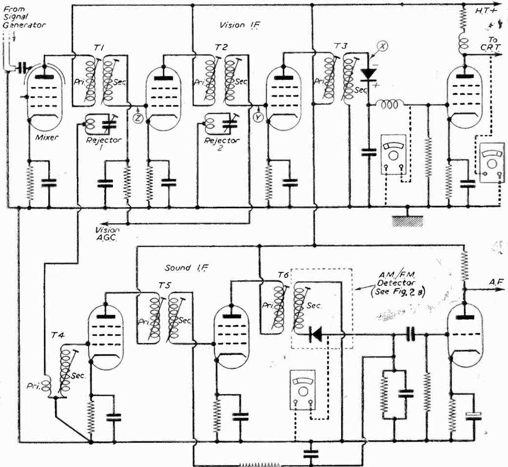
Fig. 2.—The circuit to which the text refers. (Typical but not practical.)
