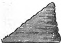
Fig. 4.—Usual form of Rubber for French Polishing.
